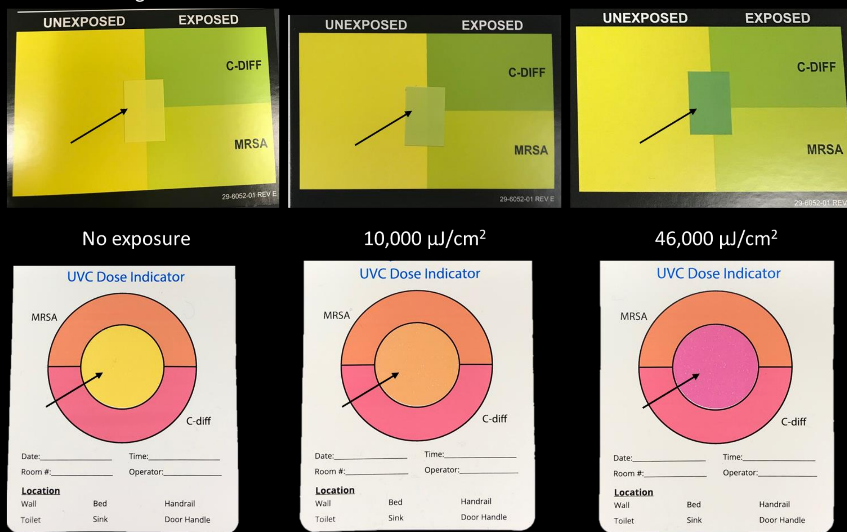
Figure 2. Interpretation of the UV indicators with UV-C dose read based on the color of the central reading window
